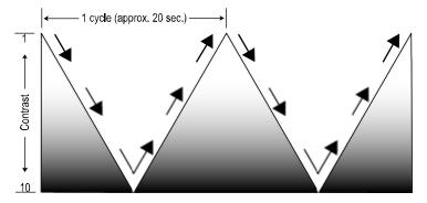
**Note:** Whenever 3sigma powers-up and the Display Control button is initially pressed and held, contrast adjusts towards the *minimum* (lightest) contrast level. Also note that whenever 3sigma first powers-up, contrast intensity is automatically set to the *last* contrast level previously used.
